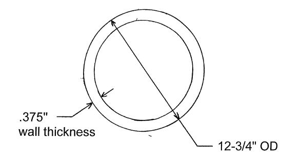
Mat'l: Carbon steel pipe ERW per ASTM A53, Grade B Material is Melted & Made in the USA
